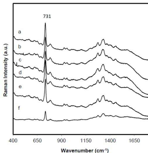
**Fig. 2** SERS spectra of ssDNA thiolated (5'SH-AAC TCG AAG TGC CAC TAC TGG C-3') sequence adsorbed from  $10^{-6}$  M concentrations obtained after (a) 20 min, (b) 60 min, (c) 2 h, (d) 6 h, (e) 24 h and (f) 7 days of storage under ambient conditions.
