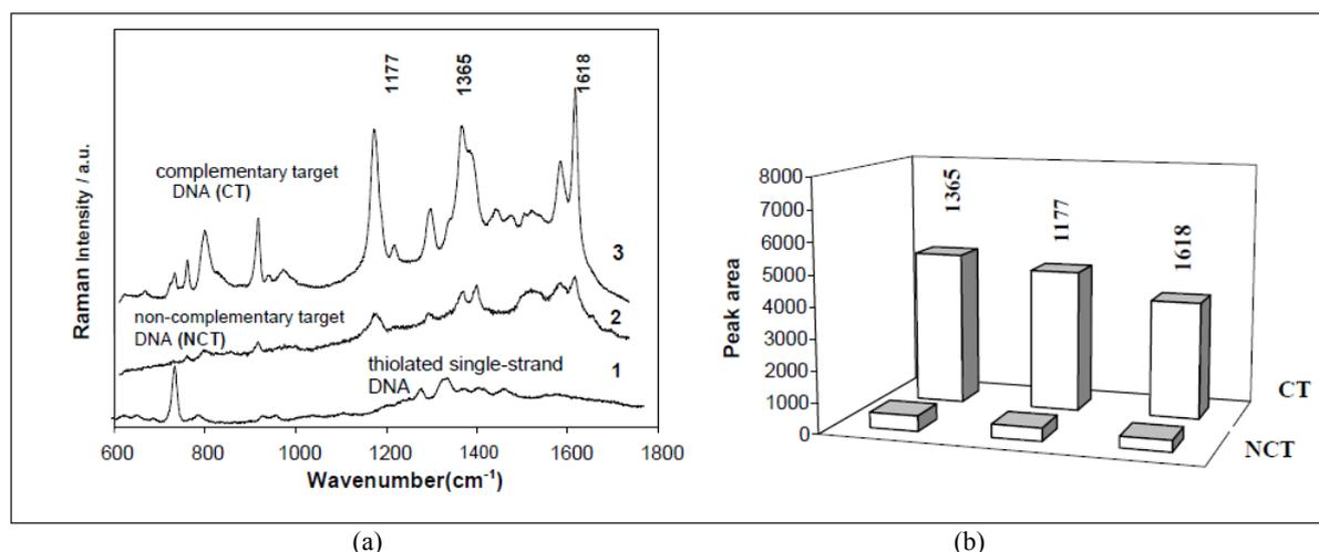
**Fig. 3** (a) SERS spectra of a surface with the thiolated ssDNA (1), a surface with ssDNA after hybridization with non-complementary DNA (Met244Val mutation) (2), and a surface with ssDNA after hybridization with complementary DNA ( $\lambda_{exc} = 632.8$  nm) (3); (b) Raman intensity of three different Raman bands at 1,177, 1,365 and 1,618 cm<sup>-1</sup> (marked in Fig. 3(a)) detected for the CT and NCT target DNA sequences, respectively.
