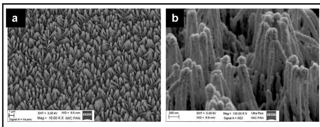
Fig. 1 (a) SEM images of a GaN platform after KSO-D photo-etching and sputtering of 70/30 % Au-Ag alloy; (b) the same surfaces after 24 h dealloying in  $\text{HNO}_3$ ; samples tilted by 45 $^{\circ}$ .
