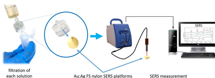
Fig. 2. The scheme presenting fast and simple preparation of a sample for SERS measurements. The syringe creates the flow of the liquid. The bacterial cells stay on the surface of the nylon mat, whereas the fluid passes through the polymer mat and filter funnel to the flask. The polymer is taken out and serves as a platform for SERS measurements.
