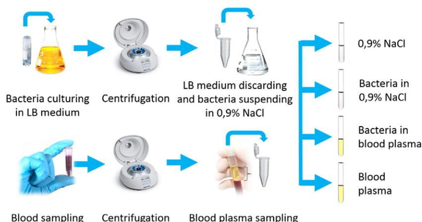
Fig. 1. The scheme presenting preparation of bacterial samples for SERS measurements.
